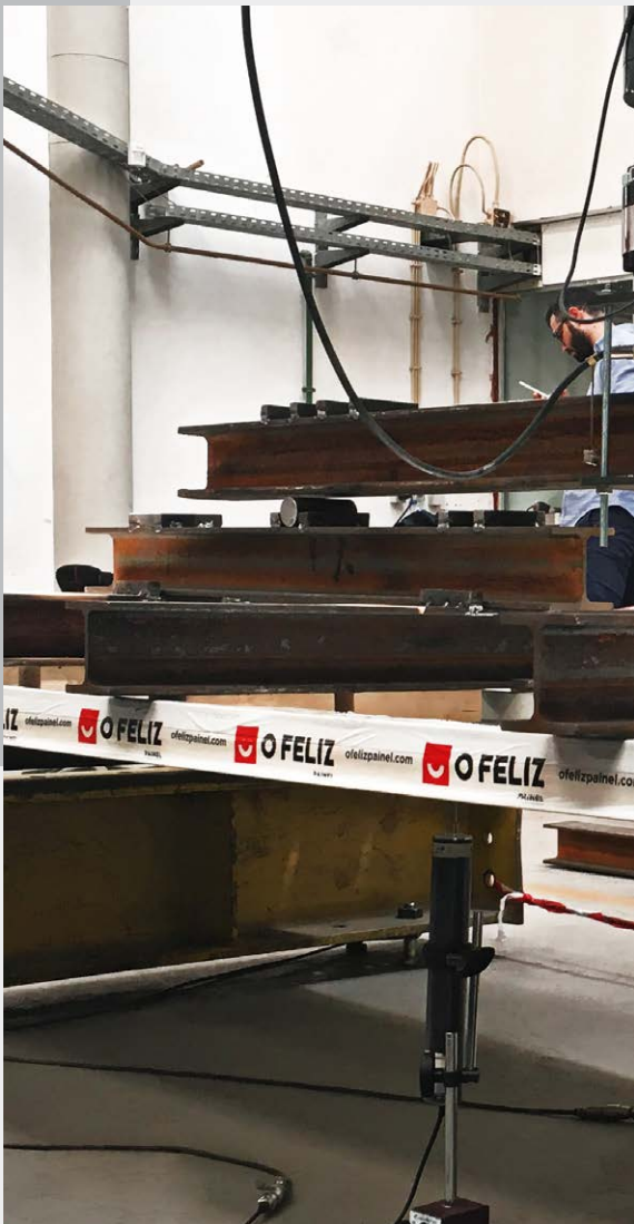
Full panel bending test
